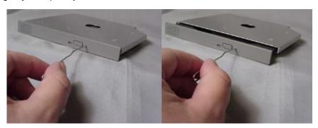
Figure 2.Using Emergency Eject
